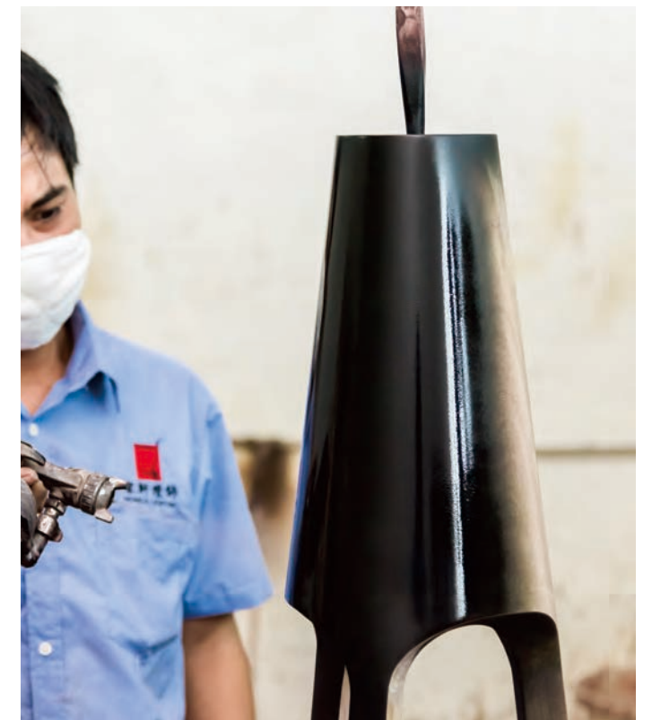
SPRAYING 喷漆涂装
